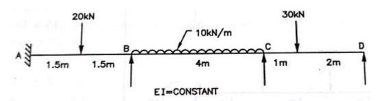
**(B)** Analyse the frame using Moment distribution method.
